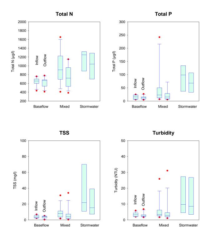
Figure 3-5. Statistical Comparison of Inflow and Outflow Characteristics for the Runoff, Baseflow, and Mixed Samples.
